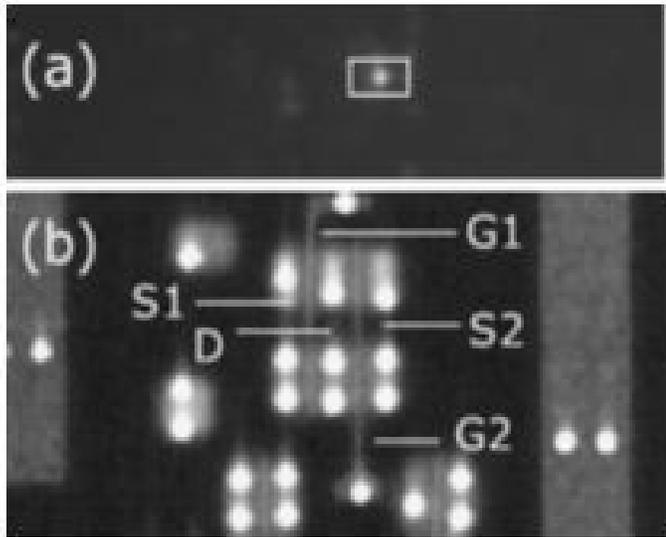
Fig. 1. (a) Image [34.84 X 270  $\mu\text{m}^2$ , L1 numerical aperture = 0.42 (50x), and working distance = 17 mm] with a single bright blob (rectangle) from two closely spaced MOSFETs, and (b) backscatter SEM image (1 X 2.2  $\mu\text{m}^2$ ) with two MOSFETs (1, 2; S = source, G = gate) sharing a common drain (D). Bright spots in SEM image are metal contacts.
