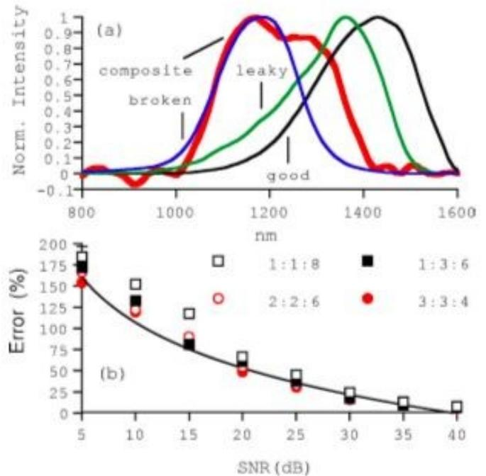
Fig. 2. (color online) (a) Composite spectrum (red, 10 nm resolution) of bright blob in Fig. 1(a), and (b) error (%) vs. SNR of composite spectrum at different power ratios of component spectra. In (a) are spectra from good, leaky, and broken MOSFETs measured with a grating spectrometer. In (b), ratio of 1:1:8 implies that good MOSFET spectrum is 8X stronger than other two MOSFET spectra. Trials per point = 9. Solid line: Error (%) = -178.8 log(SNR) + 285.7.
