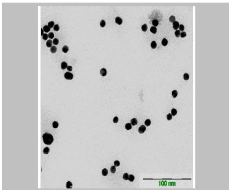
**Figure 2.** TEM micrograph of the citrate-capped gold nanoparticles.
