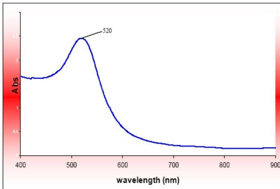
**Figure 1.** UV-Vis Spectrum of the citrate-capped gold nanoparticles.
