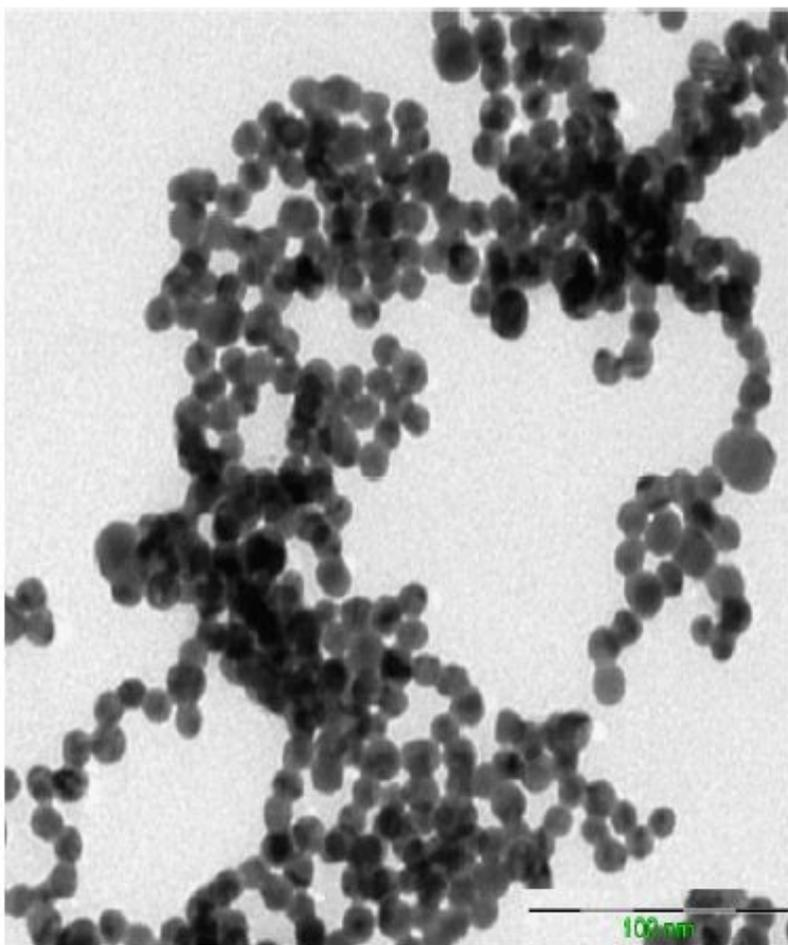
Figure 6. TEM micrographs of aggregated gold nanoparticles due to the presence of 2.5 mM  $\text{Cu}^{2+}$ .
