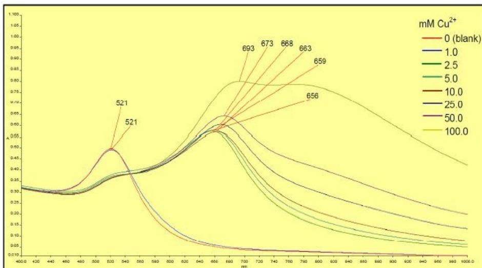
Figure 5. UV-Vis spectra of gold nanoparticles with varying concentrations of  $\text{Cu}^{2+}$
