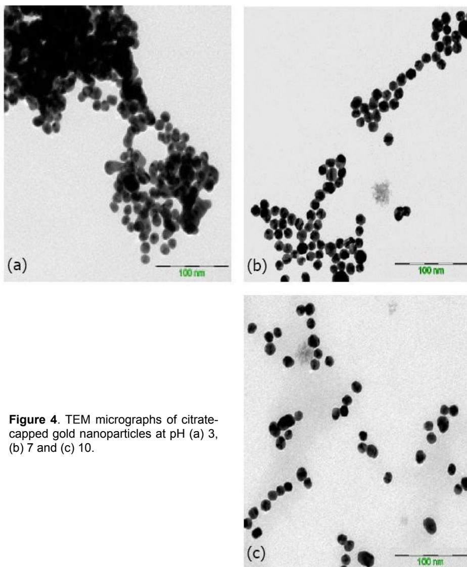
**Figure 4.** TEM micrographs of citrate-capped gold nanoparticles at pH (a) 3, (b) 7 and (c) 10.
