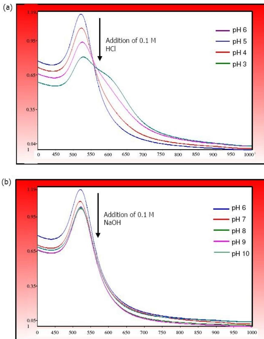
**Figure 3.** UV-Vis spectral evolution of the citrate-capped gold nanoparticles upon progressive addition of (a) 0.1M HCl and (b) 0.1M NaOH
