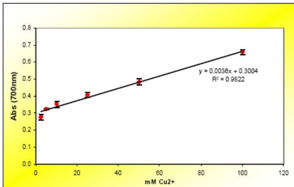
Figure 7. Calibration curve for the determination of  $\text{Cu}^{2+}$  at optimum parameters
