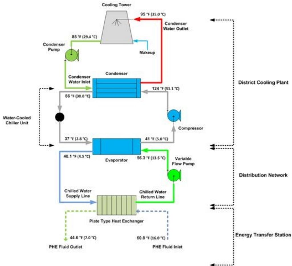
Figure 1. Overview of district cooling system with temperature limits
