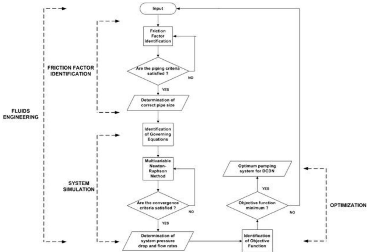
Figure 5. Logical structure of optimum pumping system for distribution network
