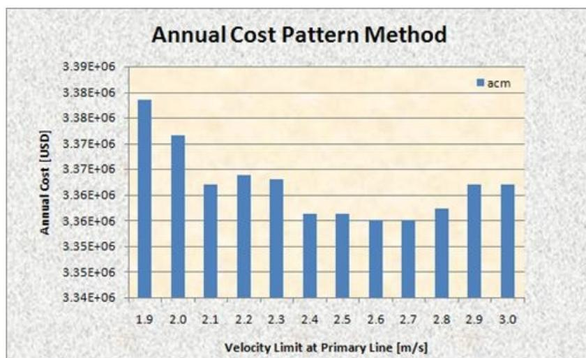
Figure 11. Optimization based on annual cost pattern method for DNModel-03\_12
