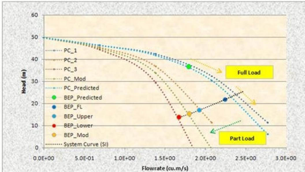
Figure 7. Best efficiency points at part load and full load conditions for DNModel-03\_12
