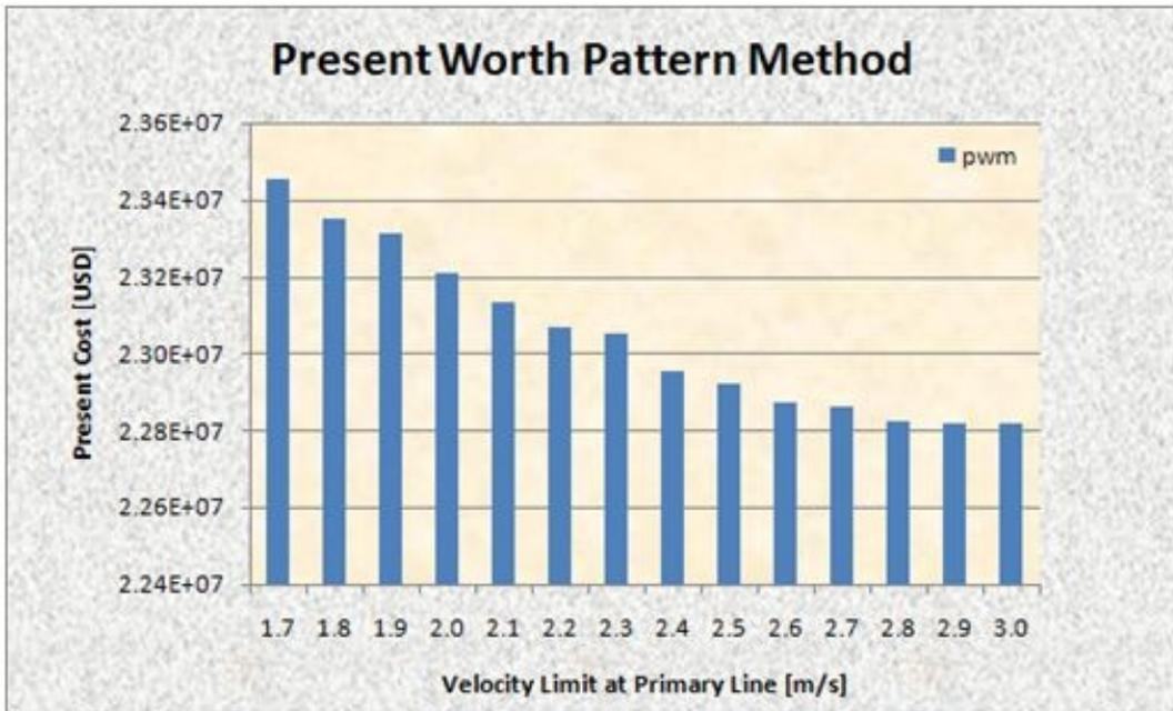
Figure 8. Optimization based on present worth pattern method for DNModel-01\_12
