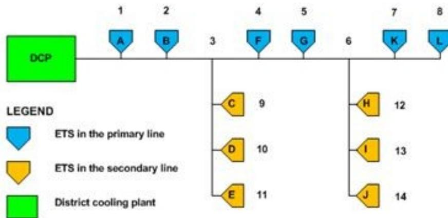
Figure 4. Schematic diagram of distribution network DNModel-03\_12
