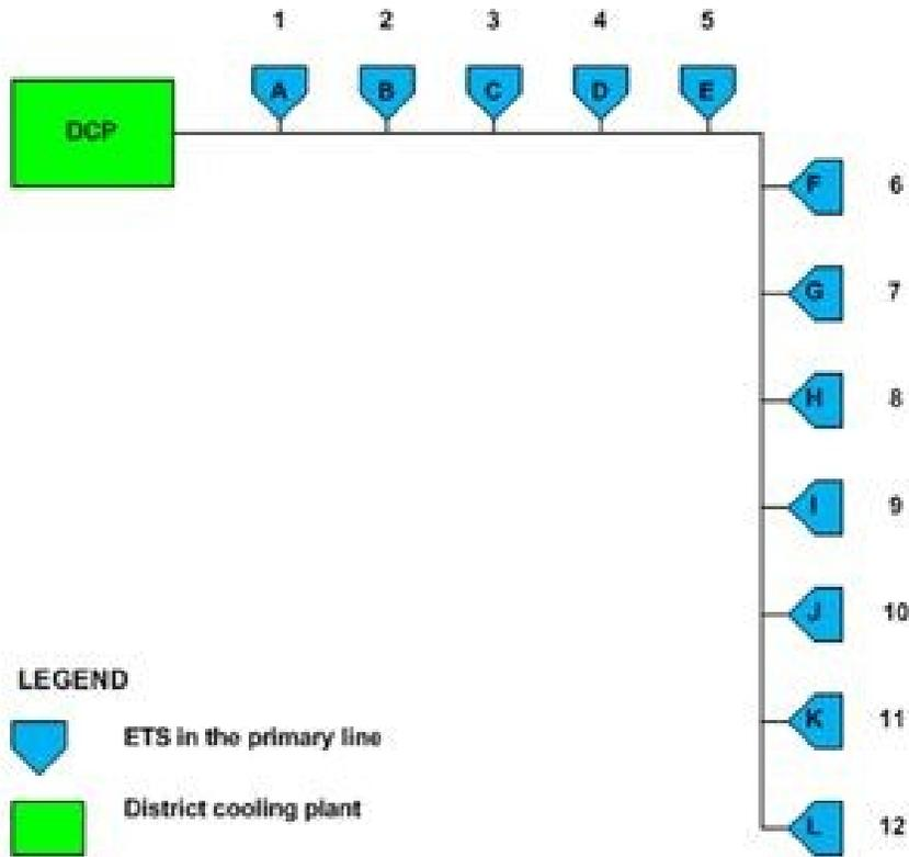
Figure 3. Schematic diagram of distribution network DNModel-01\_12
