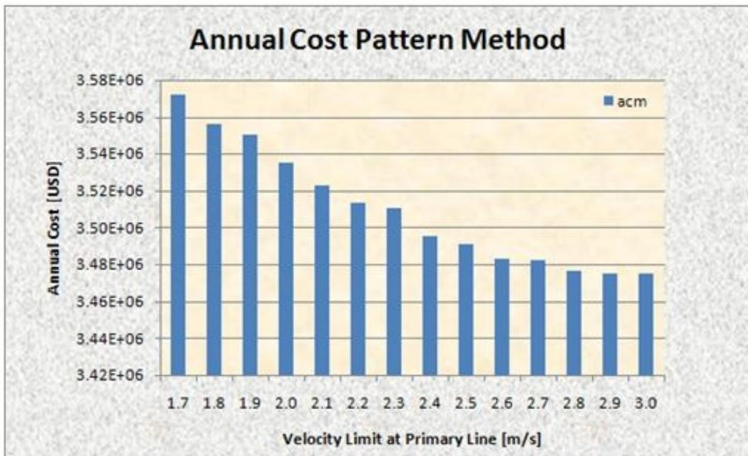
Figure 9. Optimization based on annual cost pattern method for DNModel-01\_12
