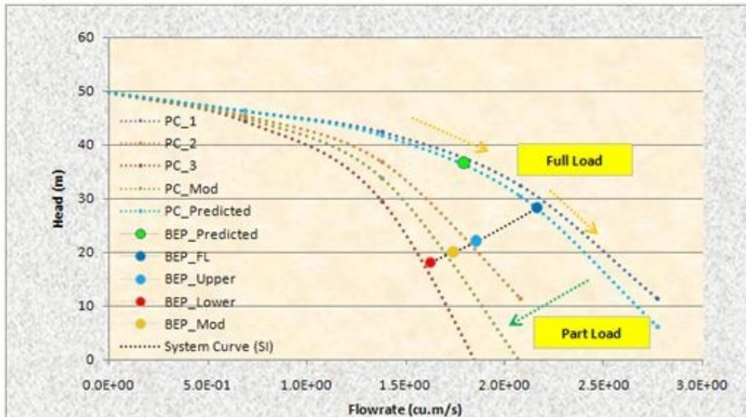
Figure 6. Best efficiency points at part load and full load conditions for DNModel-01\_12
