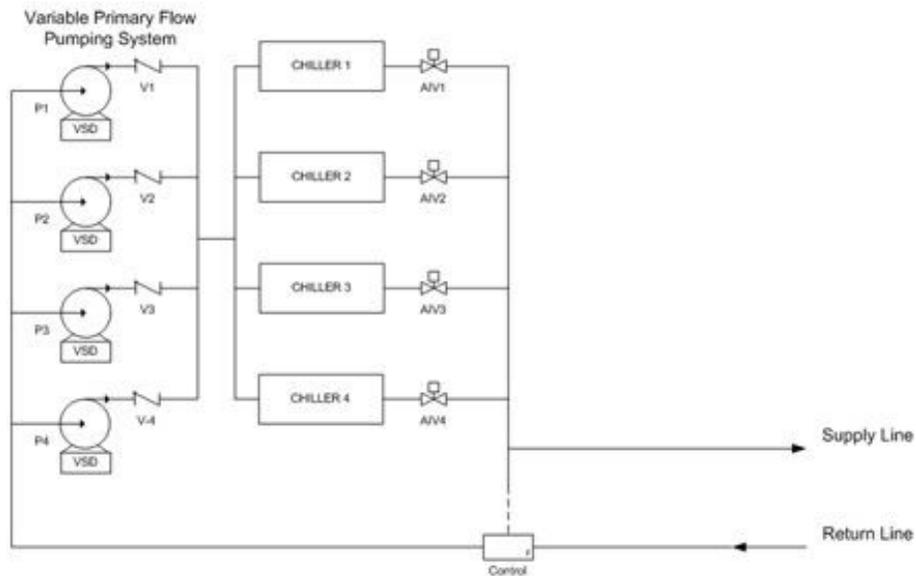
Figure 2. Variable primary flow of chilled water pumping arrangement
