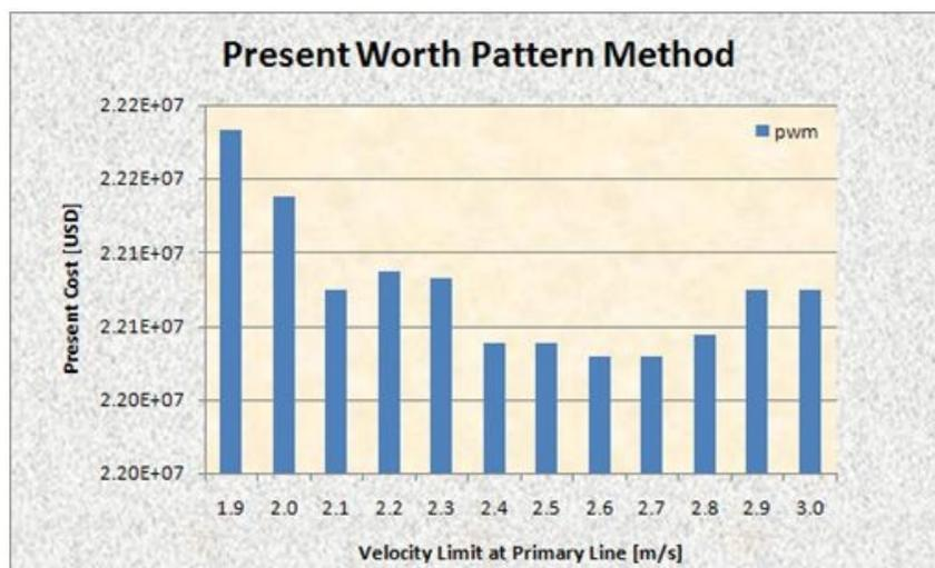
Figure 10. Optimization based on present worth pattern method for DNModel-03\_12
