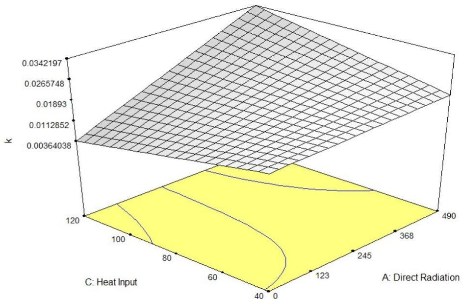
**Figure 9.** The drying coefficient  $k$  profile for air velocity of 1.9 m/s at varying direct radiation and convective heat input.
