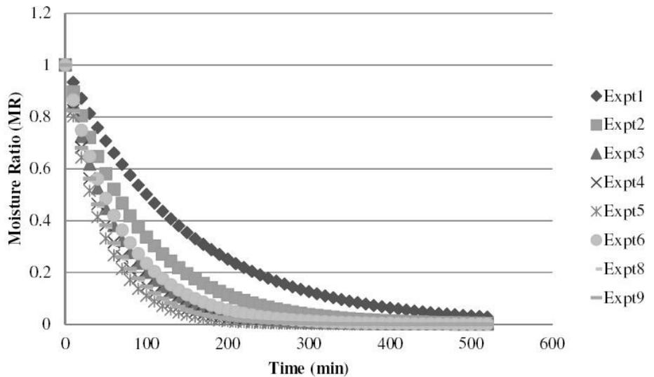
**Figure 7.** Results of curve fitting in Newton's solar drying kinetic model: moisture content versus time plot.
