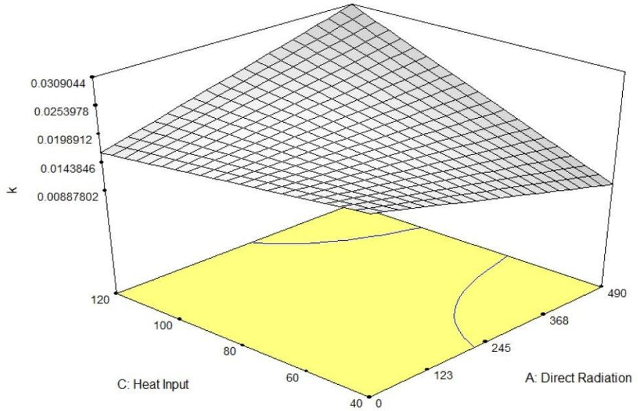
**Figure 10.** The drying coefficient  $k$  profile for air velocity of 2.2 m/s at varying direct radiation and convective heat input.
