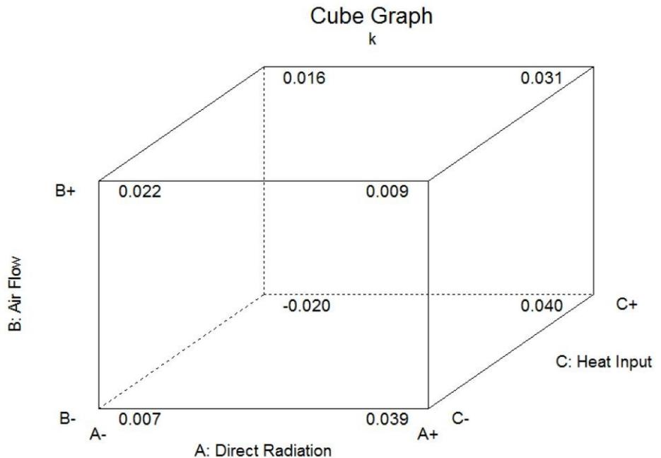
**Figure 11.** The cube graph of the drying coefficient  $k$  for the three factors: direct radiation, air velocity, and convective heat input.
