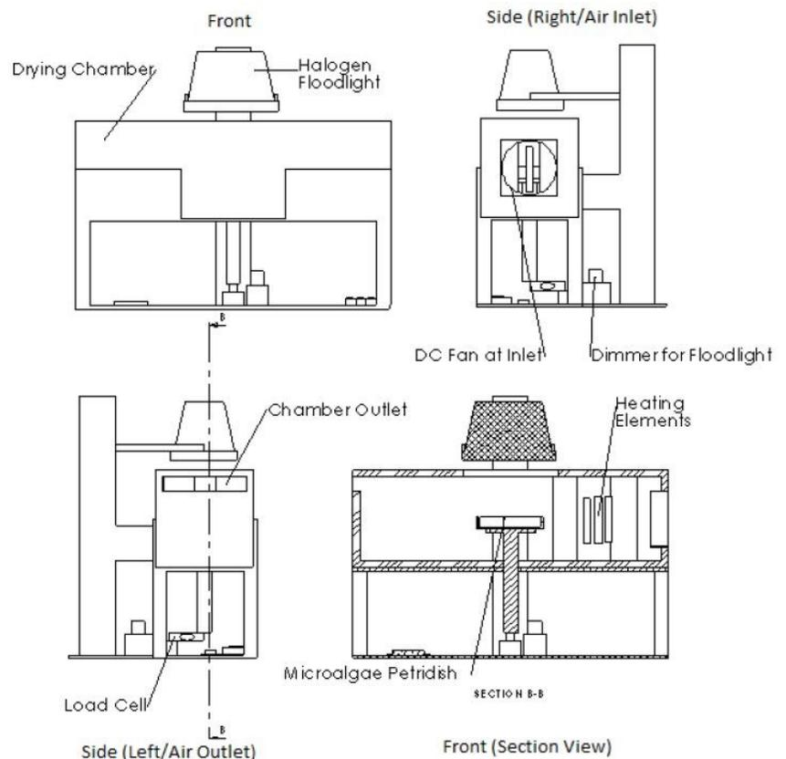
**Figure 3.** Schematic diagram of the experimental setup. Dimensions of the drying chamber: 120mm × 120mm × 450mm; Air outlet cross-section: 120mm × 20mm; Air inlet diameter: 80 mm with DC voltage controlled fan; Petri dish diameter: 100 mm. Specifications: Heating elements: 3 × 40 W; Halogen flood light, 150W, dimmer controlled; Load Cell – 1 kg max, 0.1 g sensitivity.
