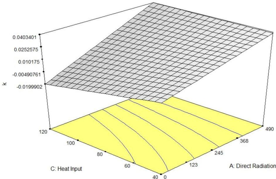
**Figure 8.** The drying coefficient  $k$  profile for air velocity of 1.3 m/s at varying direct radiation and convective heat input.
