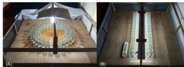
Appendix Figure 1: Growth chamber showing the light sources, and distances of test vessels from lamps in culture methods 1 (A) and 2 (B).
